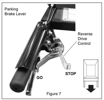
**IMPORTANT:** Avoid damage! DO NOT engage both forward and reverse control levers at the same time.
